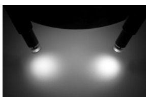
Comparison of intensity of Photonic fibre-optics with 80 LED ring light, at maximum brightness
